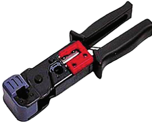
FIGURE 18.25 A combination cable stripper, crimper, and snippers
