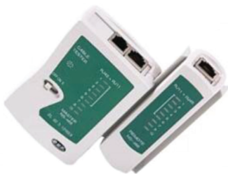
FIGURE 3.23 An inexpensive cable tester
