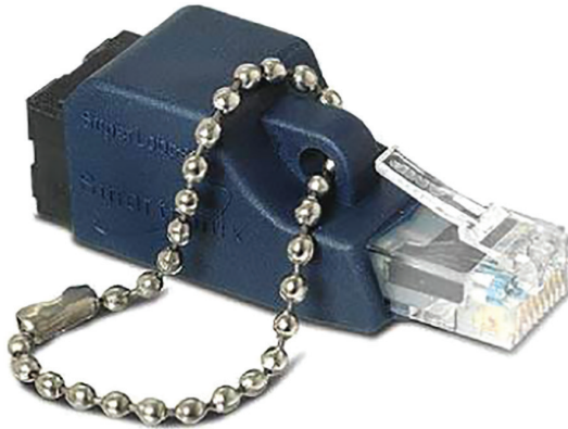
FIGURE 18.16 Ethernet loopback plug
