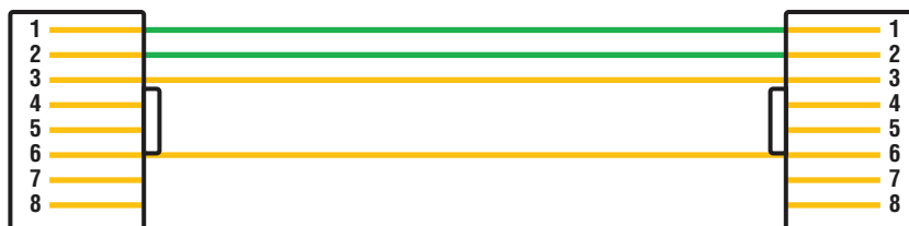
FIGURE 3.21 Straight-through Ethernet cable
